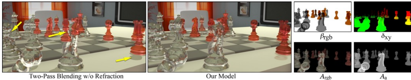
Fig. 19: A glass chess set rendered with two draw calls and naive blending vs. our method in a single draw call for all transmissive surfaces. The \delta_{xy} term is visualized as RGB color ((\delta_x + 1)/2, (\delta_y + 1)/2, 0) . Arrows point to some errors in the naive rendering. Our result corrects the ordering and captures the phenomena of colored shadows with caustics, refraction, and colored transmission. © 2015 NVIDIA
